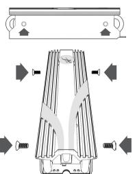
**8.** Insert the drive (with the heatsink) to your motherboard into the M.2 slot. Then insert the screw into the motherboard to hold the drive in place.
