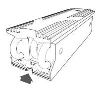
7. Align the holes that are on the side of the tray with the screw holes that are on the side of the heatsink (you may need to apply pressure). Then, insert 2 screws on each side.
